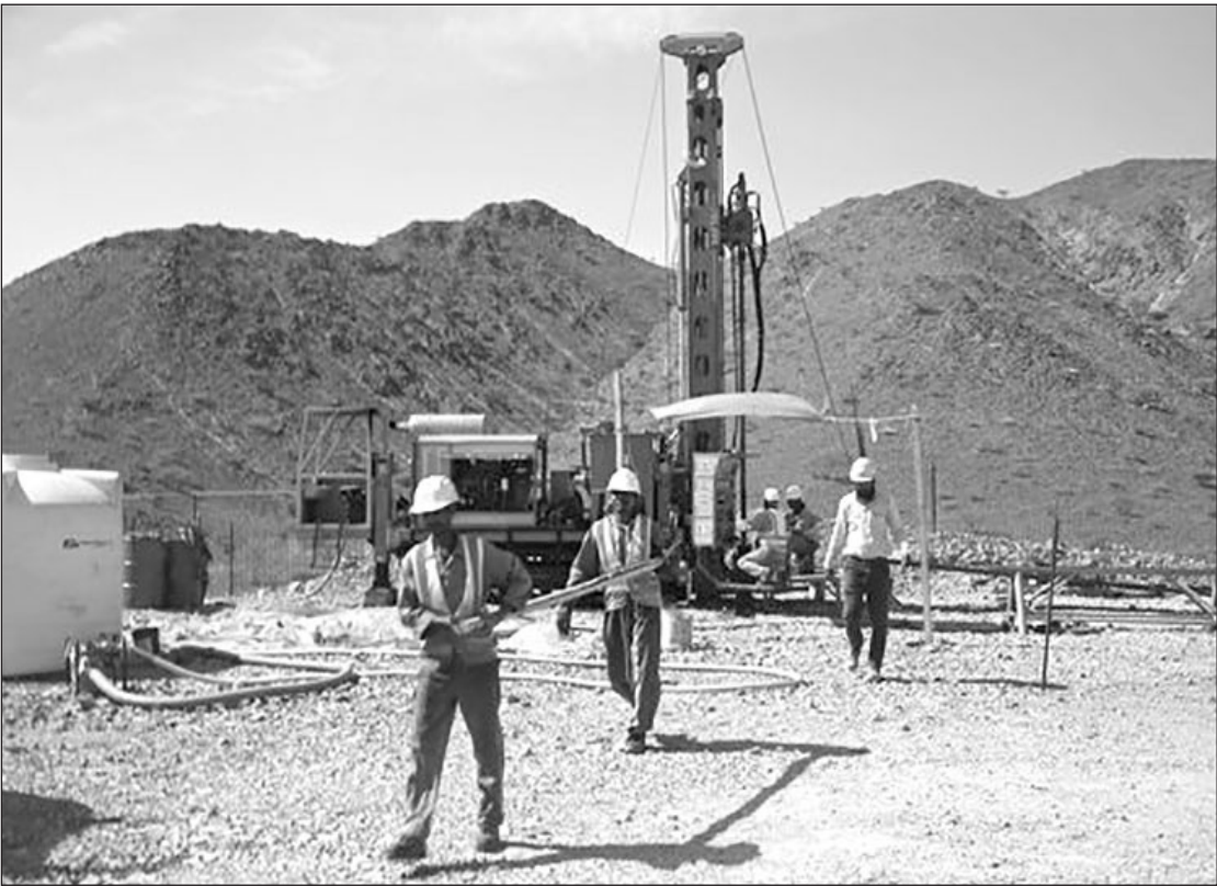
A crew removes a core sample for testing. Scientists working in Oman are searching for ways that carbon might be removed from the atmosphere and safely stored elsewhere.
